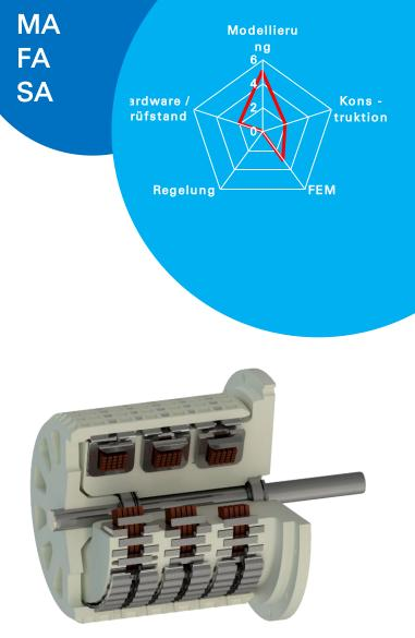
Fig. 1: Sectional view of the investigated Transverse Flux Machine
